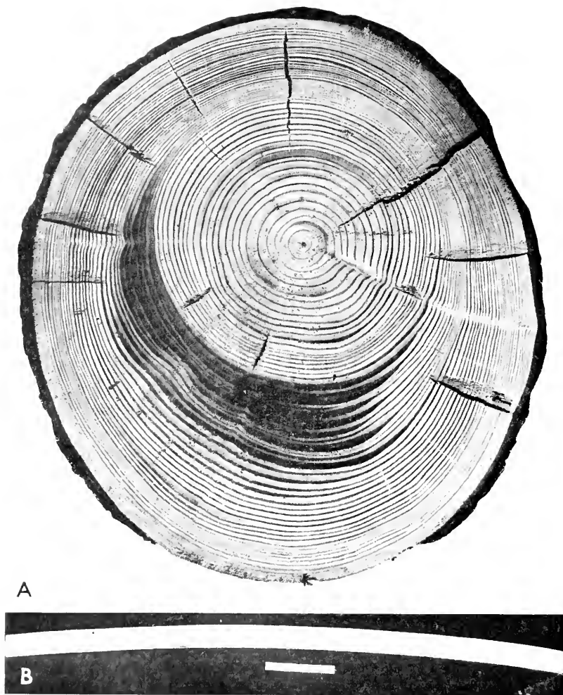
Compression wood: A, The dark, wide rings in the lower part of the cross section are compression wood; B, crook caused by the extreme longitudinal shrinkage of compression wood on the upper edge of a 2 by 4 inch stud. The 12-inch ruler indicates the length of the 8-foot stud
